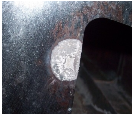
Figure 9. Aluminum buildup observed on die side face of bolster.
